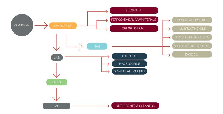
LAB: Linear alkylbenzene HAB: Heavy Alkylate bottom LABSA: Linear alkylbenzene Sulfonic Acid LAS: Linear alkylbenzene Sulfonate
