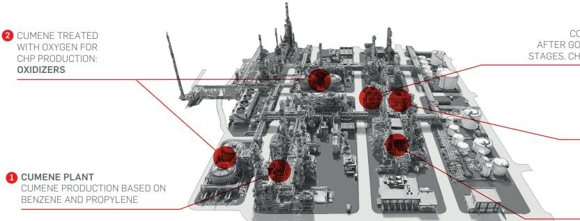
PREFLASH AND FLASH COLUMNS 3 CONCENTRATION/EVAPORATION STAGE AFTER GOING THROUGH PREFLASH AND FLASH STAGES, CHP CONCENTRATED FROM 33% TO 85%
